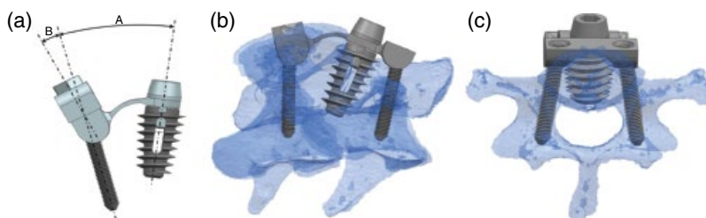
Figure 25.6 Custom fixation unit for single intervertebral fusion. Cervical Fitzateur and FITS™ (Fitz Intervertebral Traction Screw). (a) The cervical Fitzateur system comprises three elements; an intervertebral spacer (FITS device), plate and saddle. Locking screws are used to secure the saddles to adjacent vertebrae. (b) The angle of screw application is designed to maximize bone engagement, avoid incursion of the spinal canal and avoid convergence with the FITS spacer (Image a, arcs A and B). (c) Locking screws are divergent in the transverse axis and secured within the vertebral pedicle with care taken to avoid interfering with the vertebral canal and facet joints. The leading edge of the FITS device is flush but does not penetrate the ventral border of the vertebral canal (b and c).
