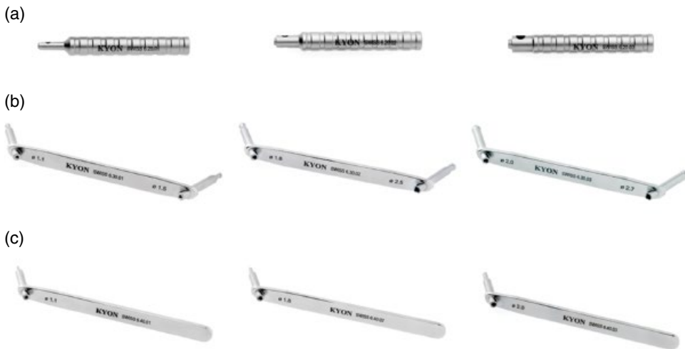
Figure 7.4 The different drill guides are shown. The guides for locking screws (a) must be held by hand in position during the drilling. (b) The guides for cortical screws allow for angulation in both planes, centering the screws in the plate hole. These guides are also used to position lag screws. The guides in the lower row (c) are used to drill the bone holes eccentrically in the plate hole and in this manner to create interfragmentary compression.
