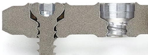
Figure 11.1 Cut-away section of a 3.5 string of pearls (SOP) plate, with screw in situ. The base is threaded to accept a standard cortical bone screw and the inner surface of the pearl features a small ridge – the aperture reduces from 6.00 to 5.85 mm diameter – against which the 6.00 mm screwhead will impinge and lock.
