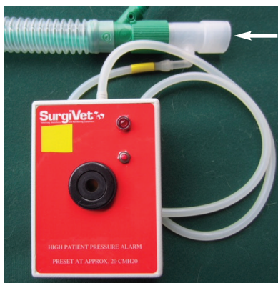
Figure 2 Example of a battery-powered high pressure alarm with an adapter (white arrow) that is inserted into the expiratory limb of a Bain NRC. Courtesy of Heidi Shafford
