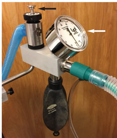
Figure 1 Bain non-rebreathing circuit (NRC) adapter with in-circuit manometer (white arrow) and safety pop-off valve (black arrow). Courtesy of Heidi Shafford
