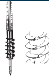
Figure 77-10. Schematic drawing of a 7.3-mm cannulated screw with the guide pin inserted and half of the shaft removed. Insert: the reverse-cutting design of threads, which facilitates screw removal after healing of the fracture.
