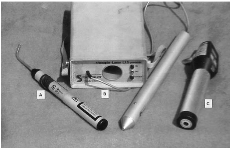
Fig. 5.15 Low level lasers: (a) CB laser (GaAs); (b) Silberaue laser (HeNe); (c) Laserex (GaAs). All these are battery powered and all are suitable for the treatment of animals.
