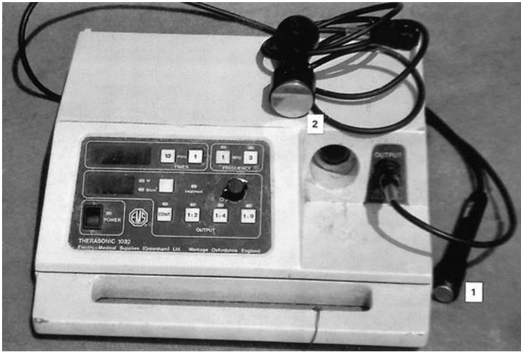
Fig. 5.8 Battery-powered ultrasound machine: (1) A small head suitable for treating tendons; (2) a larger head for treating muscle masses.
