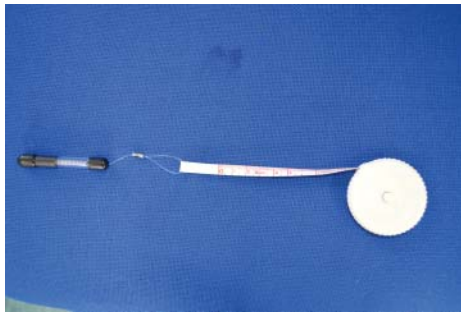
Figure 12.8 Gulicks or girthometers have a spring-loaded tensiometer device that gives more repeatable results.
