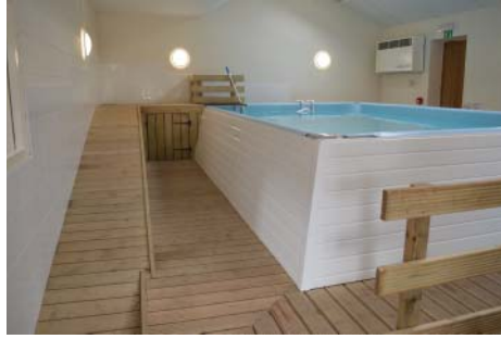
Figure 12.5 Space for even a modest pool will need careful consideration to accommodate entry and exit ramps.
