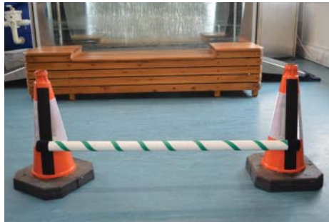
Figure 12.19 Velcro applied to traffic cones and poles provides a solid, easily adjusted system.
