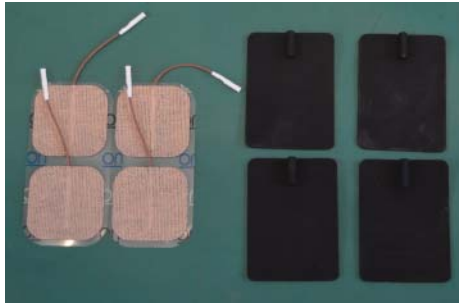
Figure 12.21 EMS pads come as disposable sticky pads or more expensive reusable rubber pads.
