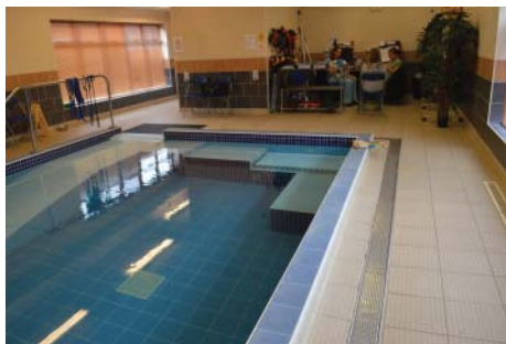
Figure 5.19 An example of a pool with submerged platforms that allow therapeutic exercises to be conducted in the warm and stimulating water environment.
