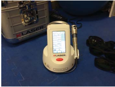
Figure 5.8 An example of a Class 4 laser. These machines have 10–20 times the power of a Class 3b laser. Safety goggles must be worn.
