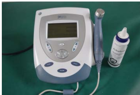
Figure 12.24 Ultrasound machine. Make sure to purchase a machine with 1 and 3.3MHz settings.
