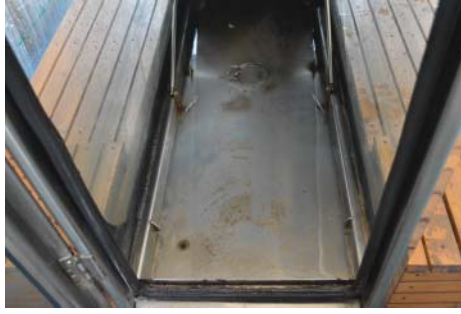
Figure 12.33 Grit from dogs' feet and grime rapidly build up in the warm watery environment of the UWTM. Try to ensure that the machine you chose can be thoroughly cleaned, even under the belt.
